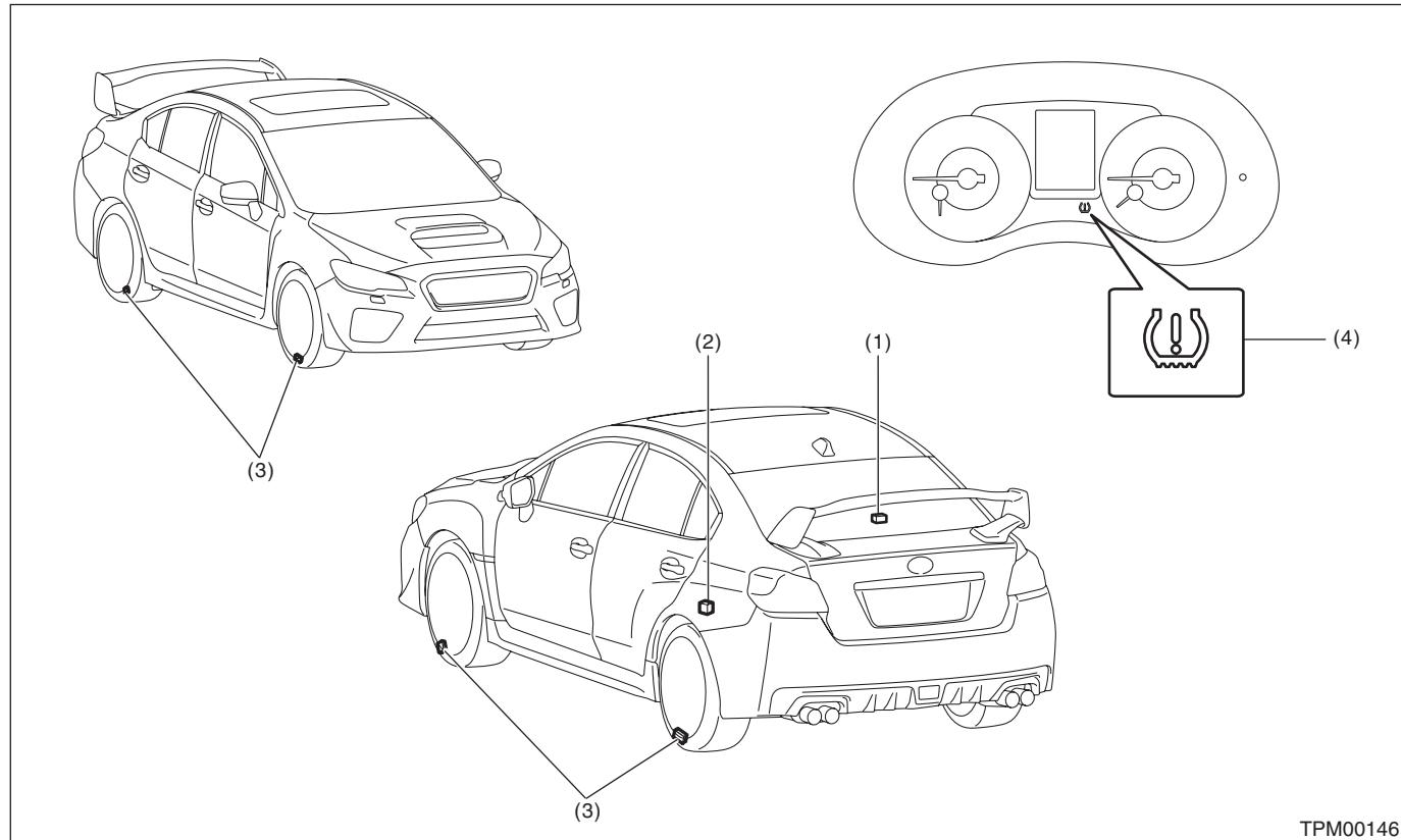
(1) TPMS & keyless entry CM (without push button start)      (3) Snap-in type transmitter      (4) Tire pressure warning light
